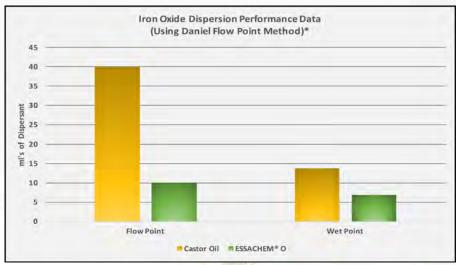
The lower the "Delta V", (The difference between the Dispersion Flow Point Volume and the Dispersion Wet Point Volume) the greater the performance of the dispersant.
